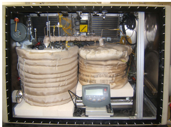
Fig. 3. Transfer of molten FLiNaK salt into the corrosion capsule inside a glove box.
